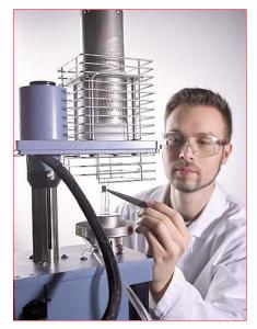
Thermal shock – shock-like temperature variations linked with the thermal expansion coefficient of materials – can lead to fractures in contacts and cables, cracks in the resin, and cause gaps to open up between the resin and plastic parts in sensitive and complex electronic and electrical components such as electronic control units and sensors.
