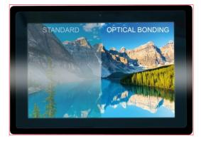
Optical bonding involves bonding two mostly transparent materials using extremely clear adhesives. The perfect coordination of process and material ensures bonding free of air bubbles. Eliminating air gaps between the joints significantly reduces refraction and improves contrast.
