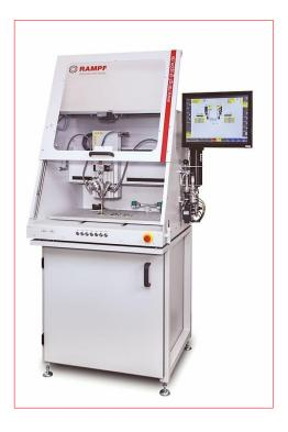
With its DC-CNC250 desktop dispensing cell, RAMPF Production Systems is presenting a cost-effective solution for high-precision dispensing of paste-like and abrasive materials. The desktop device has an integrated dispensing system and can be freely programmed for dispensing individual spots or lengths. The individual components are dispensed using a piston system designed with an extremely long service life. This results in the highest levels of accuracy and long maintenance intervals.
