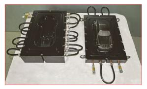
In the RTM production process, the dry fiber composite package – also called the preform – is inserted into the multi-part mold. The mold is closed and a vacuum is created. Using a mixing and dispensing system, the pressure difference then forces the epoxy infusion system via one or more injection points into the mold, which impregnates the fiber composite package. Curing times and thus the num-
