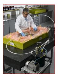
In the RI production process, the dry fiber composite package is inserted into the mold. Peel ply, flow aids, resin ducts, and vacuum channels are then put in place and the vacuum film is sealed. Once a constant vacuum has been established, the pressure difference causes the epoxy infusion system to be injected and the fiber composite package is impregnated.
