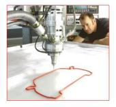
RAMPF foam gaskets are designed to comply with strict automotive industry requirements in terms of emissions and NVH standards (noise, vibration, harshness). What's more, fast-curing RAKU-PUR® Speed foam gaskets have been developed specifically for the ultrafast production chains typical of this sector – they can be ready for use within three minutes of application.
