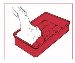
Wet cast elastomer systems from RAMPF Polymer Solutions for the production of natural stone imitations impress with their high tensile and shear strength, good chemical resistance, exceptional flow properties, very low water absorption, very low shrinkage, and excellent stability. What's more, no plasticizers are used.
