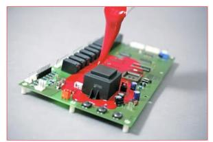
Sensitive electronic components in cars, high-precision measuring, monitoring, and regulating sensors, as well as numerous other electrical and electronic components can be reliably and efficiently protected against dust, chemical substances, and environmental influences such as heat, cold, and moisture using electro casting resins from RAMPF Polymer Solutions based on polyure-thane, epoxy, and silicone. The systems also provide a
