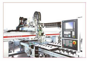
The DR-CNC dispensing robot from RAMPF Production Systems offers maximum flexibility for dynamic sealing, casting, and bonding. Variable X-Y-Z axis strokes also enable the three-dimensional application of casting, sealing, and adhesive systems. State-of-the-art control technology means the DR-CNC combines a mixing and dispensing system with maintenance-free CNC linear axes. The result is flawless interplay between the dispensing process and axis motion
