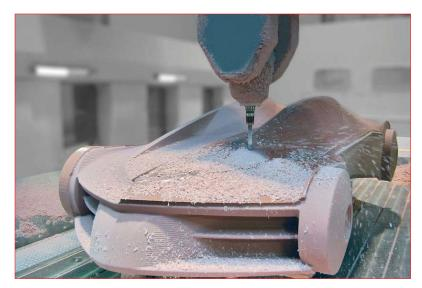
In the automotive industry, RAKU-TOOL® Close Contour Casting technology is also used for the manufacture of 1:1 size models.
