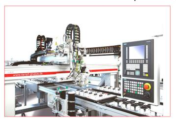
With its separate material conditioning unit, the dispensing robot offers maximum flexibility for dynamic bonding, sealing, and casting. Variable X-Y-Z strokes also enable three-dimensional material application.
