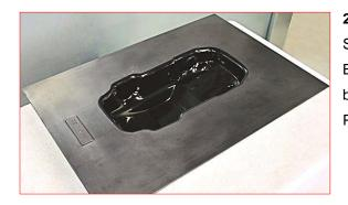
2) Prepreg shell lay-up tool, produced in resin infusion
