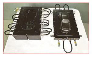
3) RTM tool (punch/ die), produced using lay-up technique
