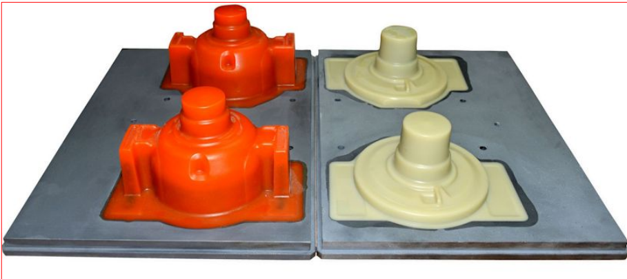
Pattern plates, produced with RAKU-TOOL ® PC-3458 / PH-3958 (left) and RAKU-TOOL ® PC-3459 / PH-3958 (right)
