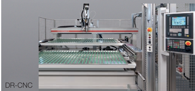
DR-CNC with side-by-side shuttle tables
