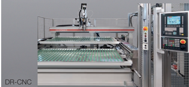
DR-CNC with side-by-side shuttle tables
