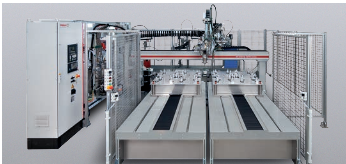
DR-CNC with side-by-side shuttle tables
