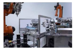
**C-DS+RA with robot and automation system** for integration into a clocked production process
