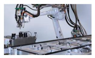
C-DS+RA with robot and conveyor belt dispensing application integrated into component production via conveyor belt system
