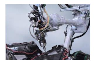
**C-DS+R with robot** for material application on complex 3D geometries
