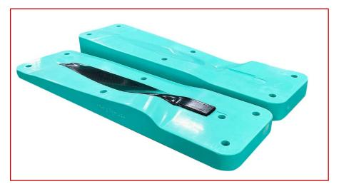
Extremely light and high-strength – the propeller blade is produced via vacuum assisted resin transfer molding (VARTM) using RAMPF's mold material RAKU® TOOL WB-0700 and high-performance liquid resins.
